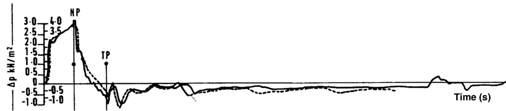
Fig. 7 Transient pressure evolution measured at 100 m from entry portal for a conventional train traveling in the Patchway tunnel [1] (NP and TP mean, respectively, nose and train passing).
